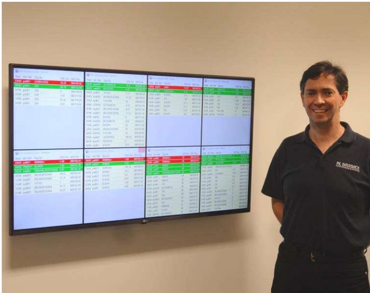
Real-time display of shop floor information highlights the current work-to-list and the jobs requiring work that day, avoiding accidental oversight of vital work. The example shown uses a T-Card style display for shop floor loading. Status Board displays can highlight which customer deliveries are due out on a particular day, allowing management decisions to be made on production as a whole. They can also warn if targets are not being met and give the shop floor priorities to focus on.
