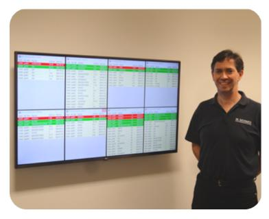
Real-time display of shop floor information highlights the current work-to-list and the jobs requiring work that day, avoiding accidental oversight of vital work. The example shown uses a T-Card style display for shop floor loading. Status Board displays can highlight which customer deliveries are due out on a particular day, allowing management decisions to be made on production as a whole. They can also warn if targets are not being met and give the shop floor priorities to focus on.
